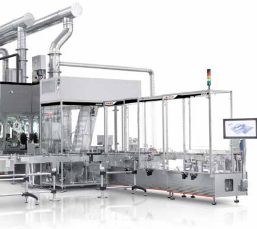
Example of Isolated Processing Line during Factory Acceptance Test activities at IMA plant
